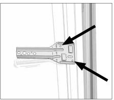
**Securing the lug in the frame.** Slip the taps into the groove and twist into place to secure a good grip. The lug can be turned free again and moved up or down to avoid any positioning issue e.g. a joint between bricks.
