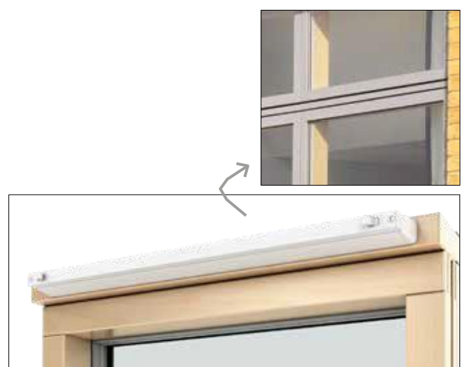
Acoustic trickle vent. The vent is machined into a timber packer with an external aluminium profile in the same colour as the window sashes. Documentation on air flow can be requested. Achieves a sound reduction value of Dn,e,w 40 dB.
