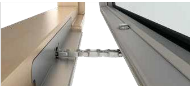
Electric opener for remote operation for windows. Can be computer controlled for fully naturally ventilated projects. Fully concealed in the frame. Three chain lengths offering 60mm, 210mm and 440mm clear opening.
